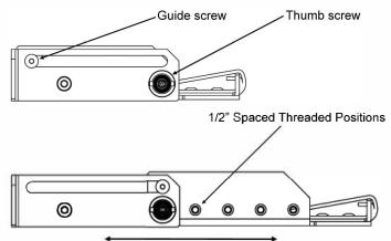
3. Install E-Z Route. After all adjustments have been made in steps 1 & 2, loosen bottom equipment bracket screws. You only need to loosen the bottom equipment bracket screws (one on each side of the equipment) to allow the E-Z Route bracket slot to slip behind the heads of the equipment bracket screws.
